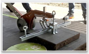
For all non - magnetic manholes covers without a hooking filled with stone or concrete), it is recommended to create a new attachment point which guarantees a secure grip by means of the opening devices. The lasting transformation makes the opening operation easy and regulatory-compliant.
