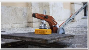
The Rhino Slim Dumped magnet does not require power supply, allows **you to perform interventions quickly** without renouncing safety, it frees the operator from the search, cleaning and use of the hooking points placed in the manhole covers.
