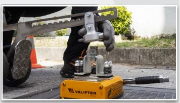
The Rhino Slim Dumped magnet integrates the unified quick coupler, making the magnet compatible with any **VALIFTER** lifting system.
